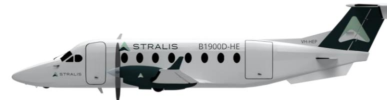
The Stralis B1900D-HE delivers reliable high performance without the carbon emissions. Stralis is modifying the renowned Beech 1900D, replacing the turbines and jet fuel system with our state-of-the-art SPS-1 Hydrogen Electric Propulsion System (HEPS) and liquid hydrogen storage tank. Aircraft features include:
